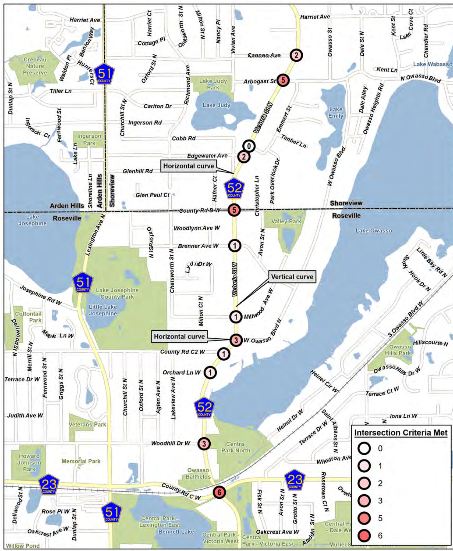
Figure 21 - Intersection Screening Results and Geometric Issues
