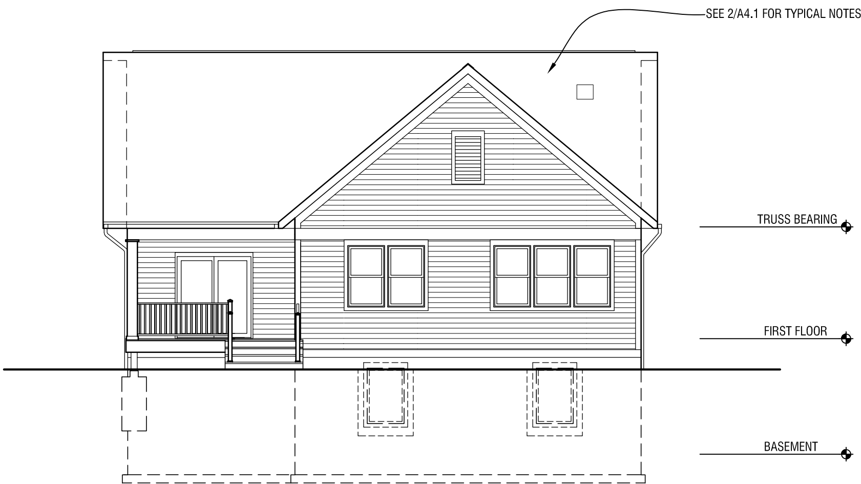
5 EXTERIOR REAR ELEVATION - SINGLE FAMILY HOME 1/8" = 1'-0"
