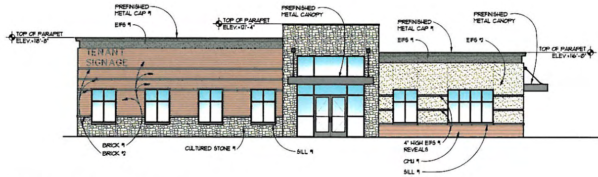
7 NORTH ELEVATION A3.1 1/8"=1'-0"
